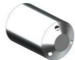
F0060006 Ø16x25; G1/4" Brass, Nickel-plated 3 Bore Holes
