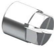
F0060001 Ø16x19; SW14; G1/4" Brass, Nickel-plated Cross Slots, broad
